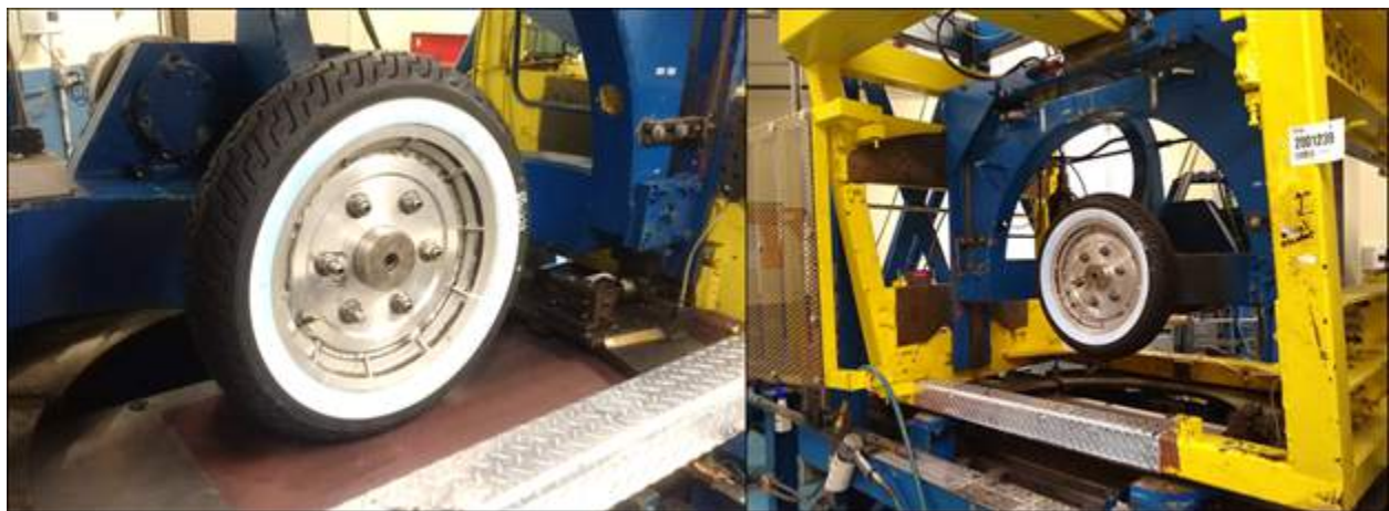
Fig. 27 Testing of the motorbike tire at Smithers facility.
