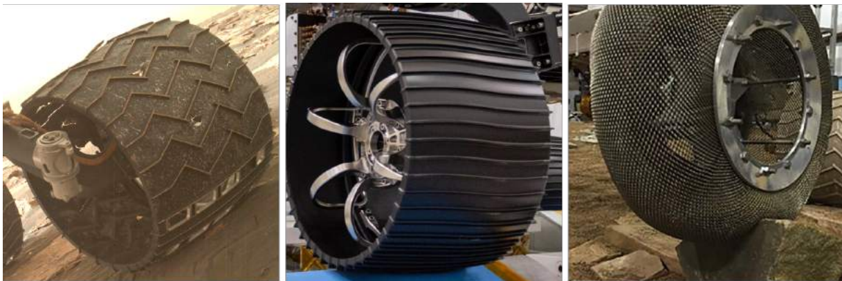
Fig. 16 State of the art in rover wheels at NASA. (a) The left middle wheel of MSL rover image taken by Mars Hand Lens Imager (MAHLI) of MSL. The holes on tire surface and broken tread on top are conspicuous. Credit: NASA/JPL/PIA21486. (b) Mars 2020 rover wheel with increased tread count and modified curvature. Credit: NASA/JPL/PIA23269. (c) The "Spring Tire" made from nickel titanium SMA undergoing durability testing in simulated Mars terrain at JPL. Credit: NASA/Imaging Technology Center at NASA Glenn.
