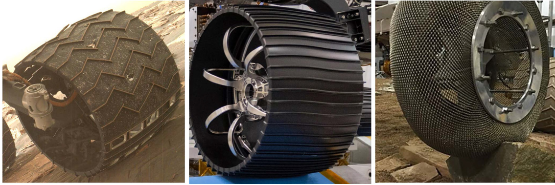
Fig. 18. Left to right: (a) Damage on the rigid Curiosity rover wheels. (b) Mars 2020 rover wheel with modified grouser pattern. (c) Compliant shape memory alloy wheel baselined for the MSR sample fetch rover undergoing obstacle tests at NASA Glenn Research Center.
