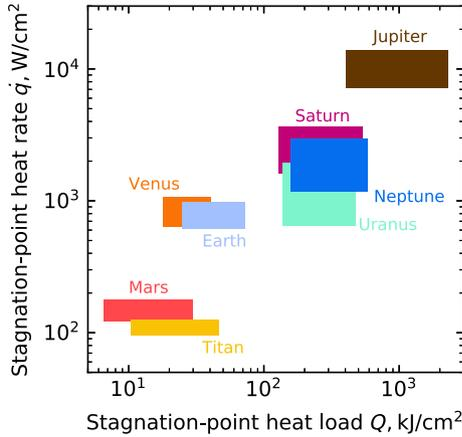
**Fig. 18** Comparison of stagnation-point heat rate and total heat load for aerocapture at various targets. Results for a lift modulation vehicle with  $L/D = 0.30$ , and arrival  $V_\infty$  range listed in Table 7.
