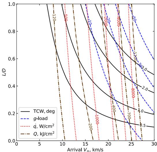
**Fig. G1 Lift modulation aerocapture feasibility chart for Uranus.**
