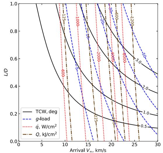
**Fig. H1 Lift modulation aerocapture feasibility chart for Neptune.**
