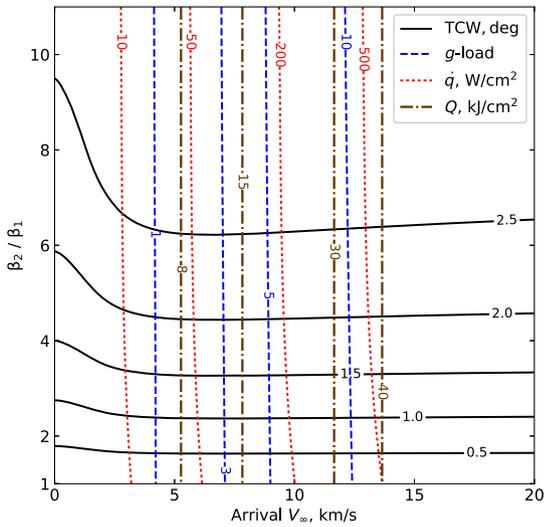
**Fig. F2 Drag modulation aerocapture feasibility chart for Titan.**
