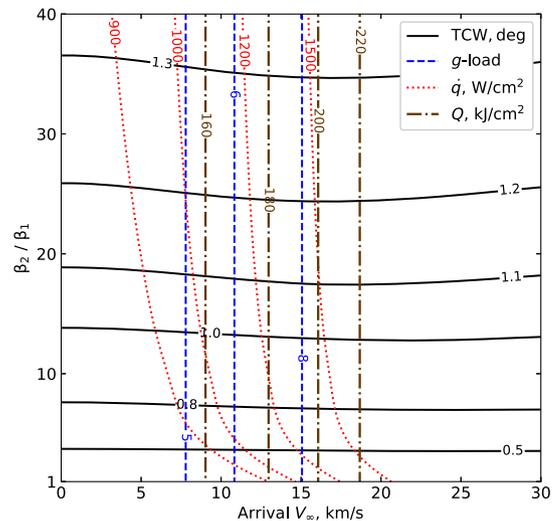
**Fig. H2 Drag modulation aerocapture feasibility chart for Neptune.**
