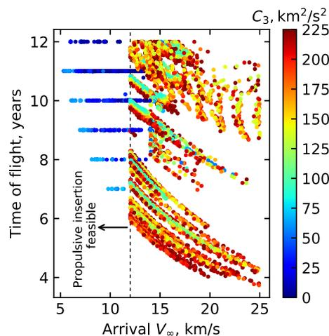
Fig. 5 Trade space for Neptune interplanetary trajectories.
