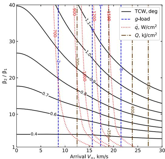
**Fig. G2 Drag modulation aerocapture feasibility chart for Uranus.**
