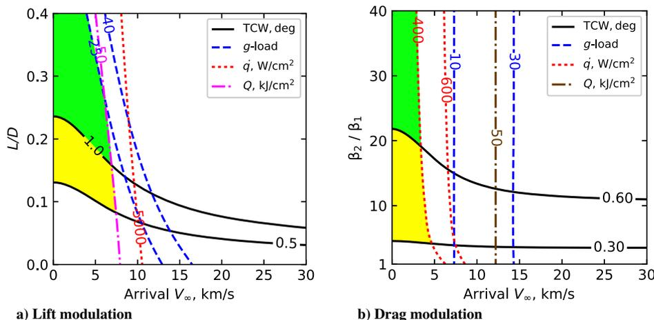
**Fig. 6** Aerocapture feasibility charts for Venus. The green region in the left figure indicates the feasible ( $L/D, V_\infty$ ) for lift modulation aerocapture with a TCW requirement of 1 deg. With a required TCW of 0.50 deg, the yellow region also becomes feasible.
