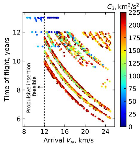
Fig. 4 Trade space for Uranus interplanetary trajectories.
