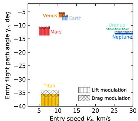
Fig. 15 Comparison of planet-relative entry speed and entry corridor for aerocapture at various targets for a vehicle with  $L/D = 0.30$  for lift modulation and  $\beta_2/\beta_1 = 7$  for drag modulation.
